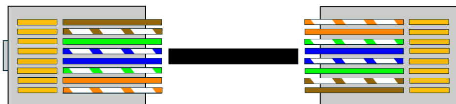
STRAIGHT NETWORK CABLE SCHEME
